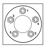
14. Tighten the wheel nuts firmly in a crisscross sequence, as shown, with the wheel wrench.
